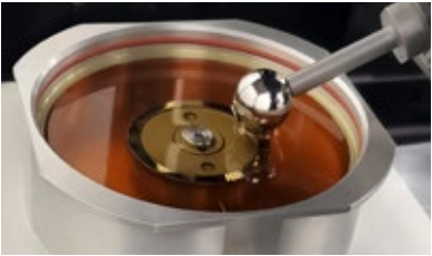
Traction Module and Sensor During a Test
