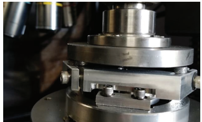
Figure 2. Brake Material Screening Setup on MFT 5000
